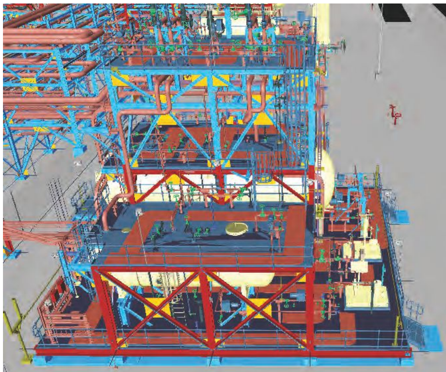
Figure 1: 3D Model of a process module for an onshore plant. Note the extent of detailing that has been carried out.
